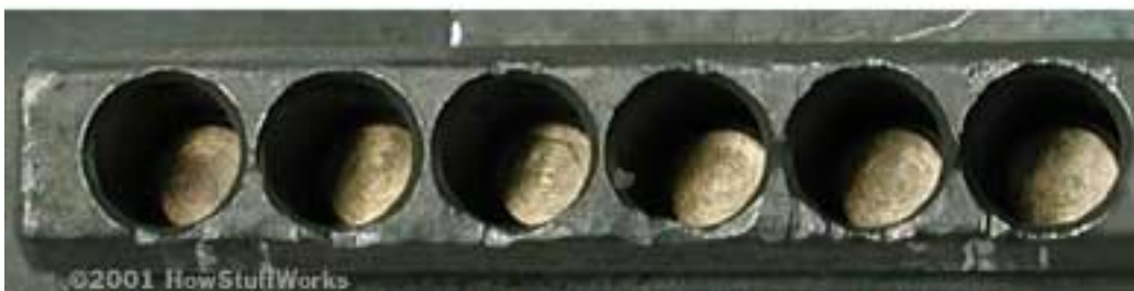
The pins in a pin-and-tumbler lock when no key is inserted (top) and
